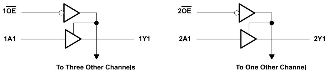
Figure 3. Logic Diagram (Positive Logic)
