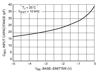
Figure 6. Input Capacitance
