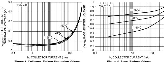
Figure 3. Collector-Emitter Saturation Voltage
