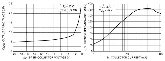
Figure 7. Output Capacitance
